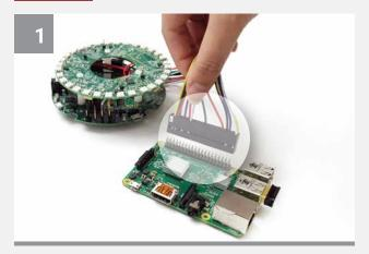
Connect the cable assembly to the GPIO pins on the RPi 3. Align the sticker labeled '1' with physical pin 1 on the RPi 3.
