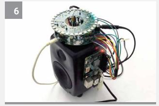
The unit should be placed on top of the speaker and affixed with some putty or foam to minimize vibrations from the speaker.
